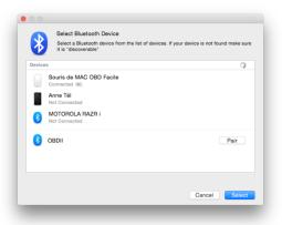
Click on « Pair », if you fail to pair, you may should change the option and tap the PIN code: 1234. When you are paired to the device, select it and click on the select button at the bottom right of the window.
